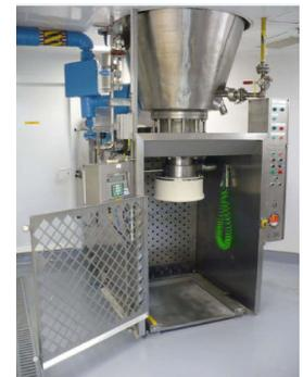
The material transfer is enclosed with the receiving vessel being docked or sealed to the source vessel.
