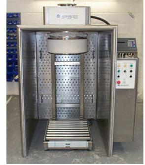
In a downward laminar flow booth, a curtain of descending laminar air flow is created between the ceiling and the rear of the booth where exhaust grills are located in the lower section. The booth contains the source and has maximally one side open..
