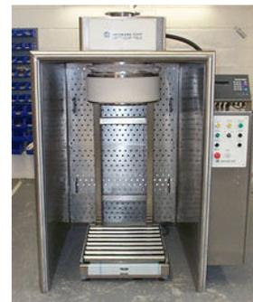
Other enclosing hoods      Any form of permanent encapsulation or encasing of the source of which maximally the front side is open with a proper local exhaust ventilation system.      0.1
