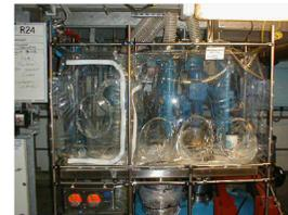
which allow products to be handled in a contained way without exhaust ventilation.
